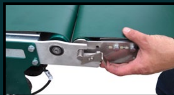
Conveyor to conveyor interlocking system
